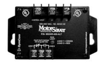
**Model 50R-400-ALT** alternating relays are used to alternate between two loads, most commonly in duplex pumping and compressor applications to balance the runtime of both loads.
